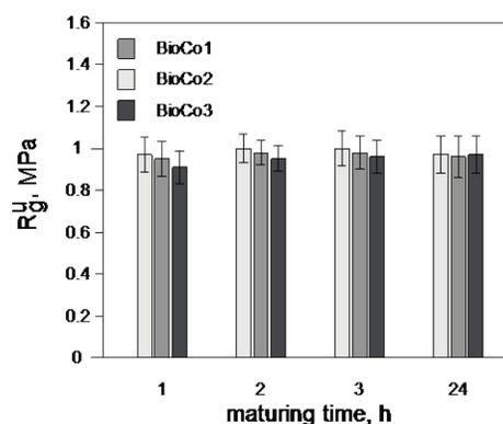
Fig. 4. Results of flexural strength measurements of sand samples bonded with BioCo binders hardened thermally
